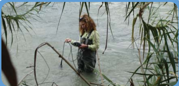
IBWC staff from Amistad Dam use a multiprobe instrument to collect field parameters such as pH and DO, downstream of Eagle Pass, TX, November 2009
